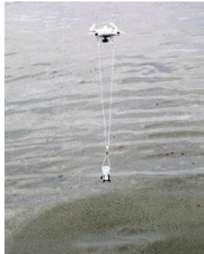
Self-designed water samplers for drone in collecting water samples at remote locations
