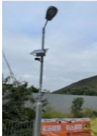
AI surveillance camera system in assisting the evidence collection for prosecution of illegal waste disposal
