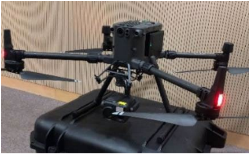
Smart drones with high zooming power camera in surveilling illegal landfilling activities
