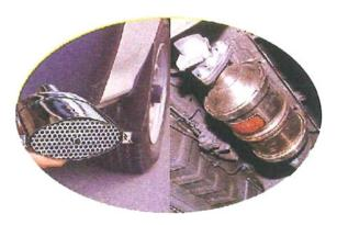
Particulate traps and catalytic converters help reduce emissions from diesel engines
