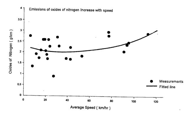
Figure 6.6 Variations in Vehicular Emissions with Speed (Source New Civil Engineer, June 1995)
