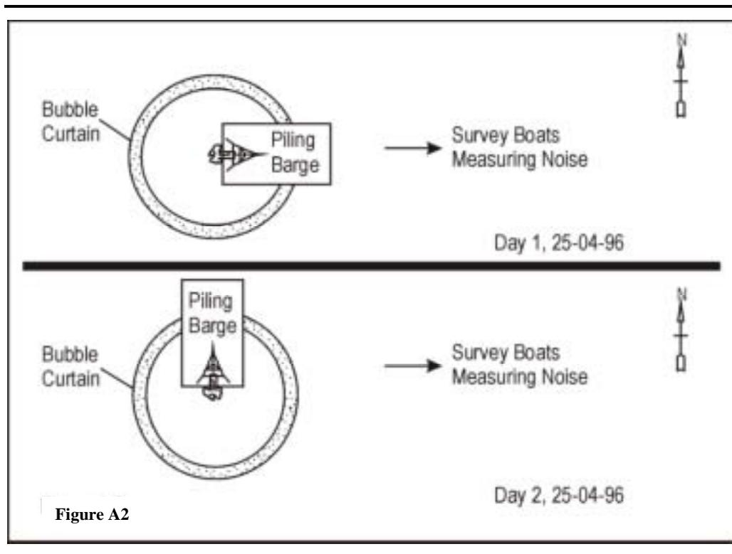
A.3. Results indicated that when the barge was not in the sound propagation path, a reduction of 3 to 5 dB was achieved in the overall broadband levels and up to 20 dB in the one octave band of 1.6 to 6.4 kHz.
