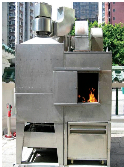
Fig.3: An example of joss paper furnace adopting BAT for emission control.
