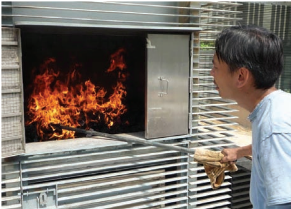
Fig.7: It is essential to employ trained operators to control the feeding rate of joss paper to the furnaces, especially during festive days.
