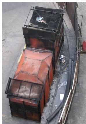
Fig.2: Typical metal paper artifacts furnace with water spraying.
