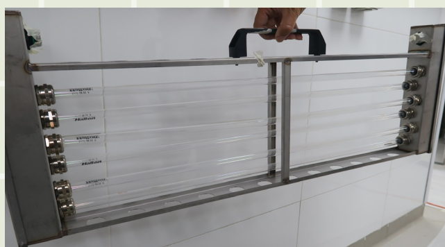
Cassette panel mounted with UV-C lamps
