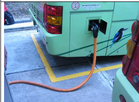
Electric bus with charging cable connected
