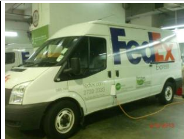
EV charging from the charging socket
