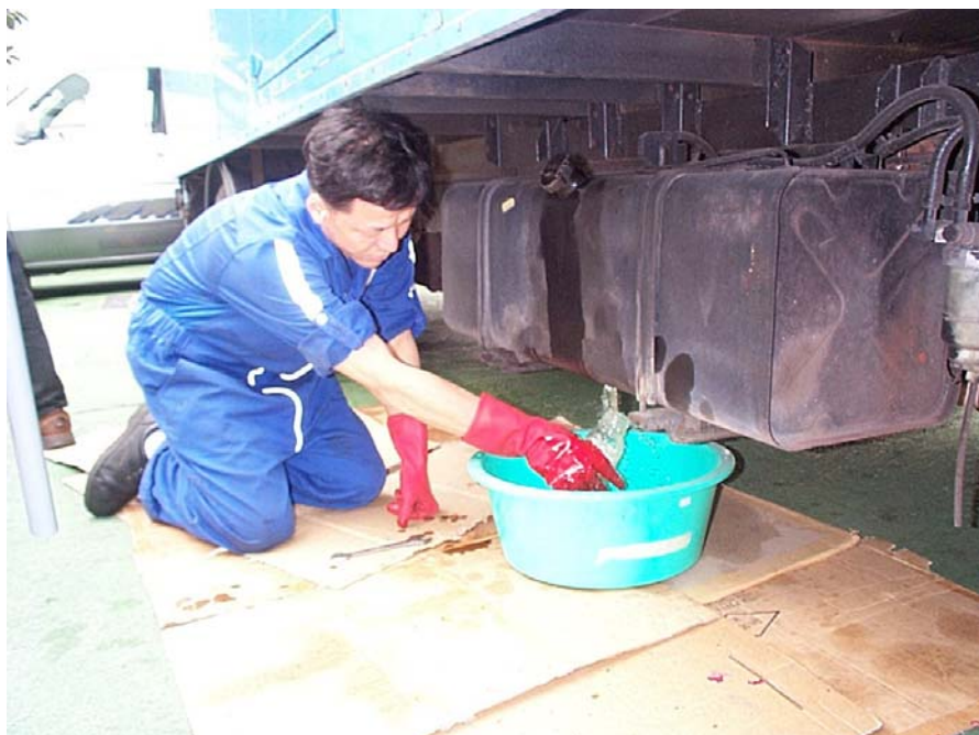
Photo 2. Change fuel at Pokfulam Fire Station (Main dynamometer test)
