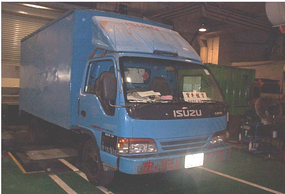
Photo 10. A test vehicle on the chassis dynamometer under the diesel lug down test (On-road performance test)
