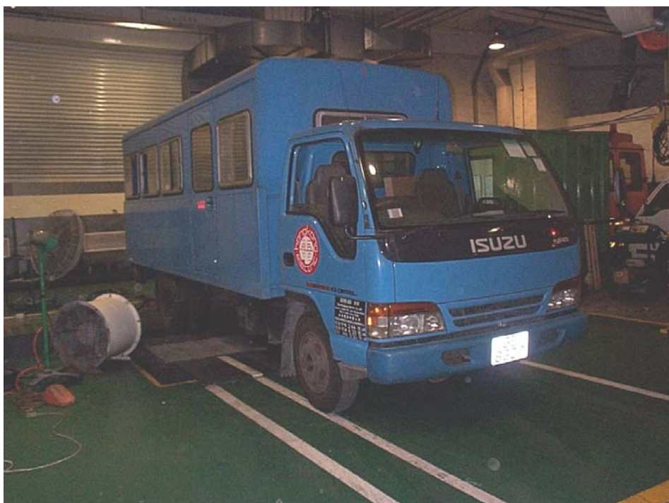
Photo 1. Chassis dynamometer vehicle exhaust emission test (Main dynamometer test)
