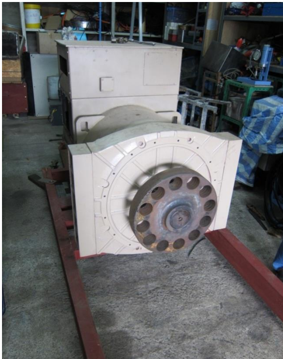
Photo 4.11. AC alternator with mechanical coupler
