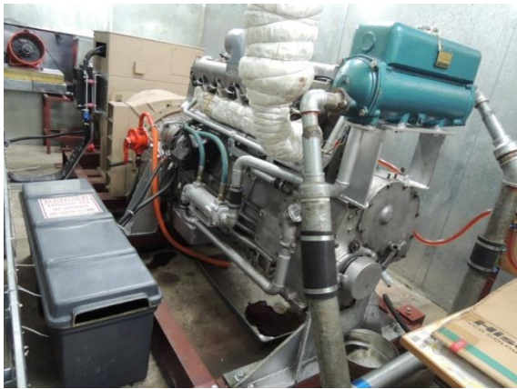
Photo 4.3. The Gardner engine installed on the test rig
