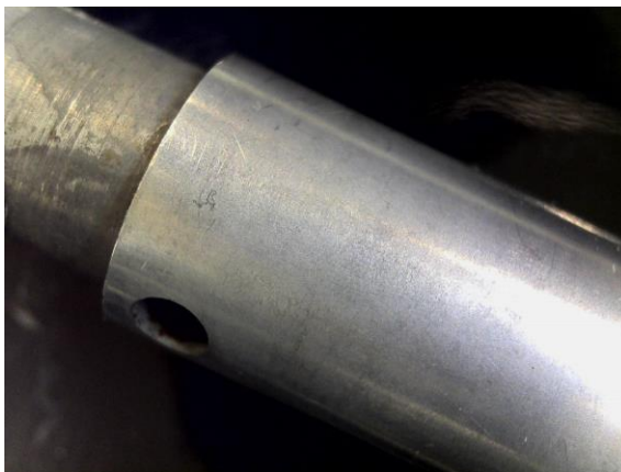
Photo 6.16. Zoom up view of the fuel metering pump plunger (Before LSD trial)
