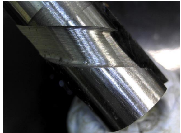
Photo 5.9. Zoom up view of the fuel pump plunger (After HSD trial)
