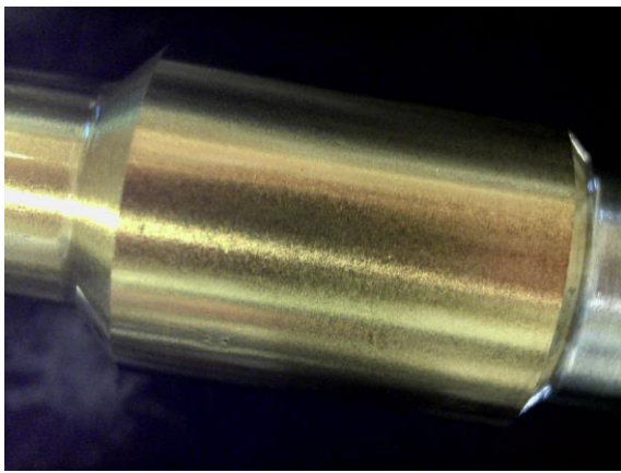
Photo 6.8. Zoom up view of the fuel injector plunger (Before HSD trial)
