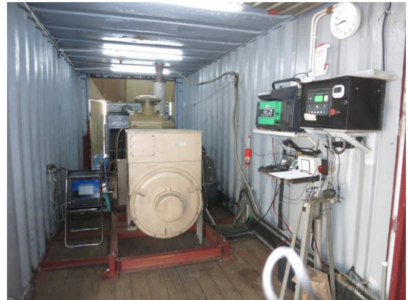
Photo 4.8. The test rig was placed in a 20-feet container
