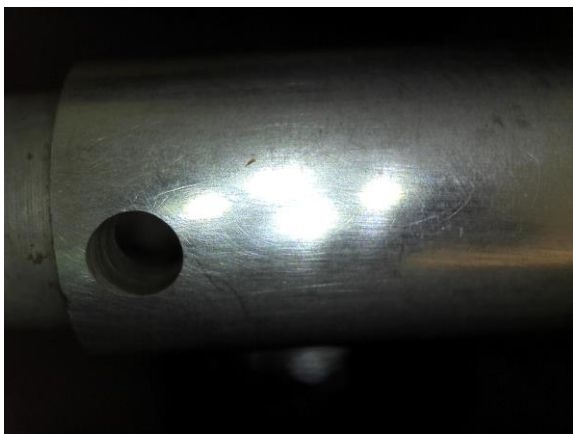
Photo 6.10. Zoom up view of the fuel metering pump plunger (Before HSD trial)
