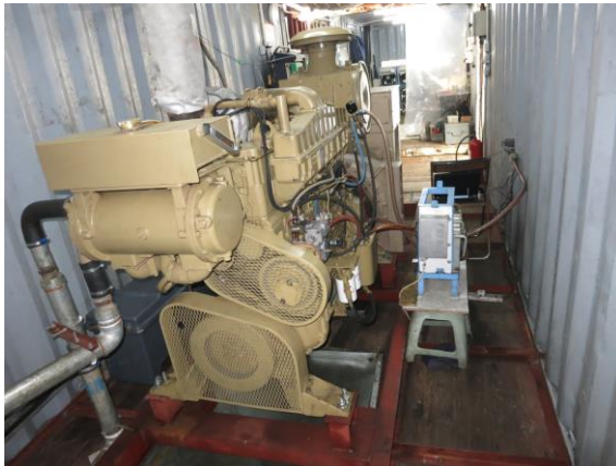
Photo 4.7. The Cummins engine installed on the test rig
