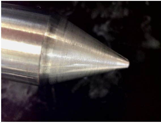
Photo 6.6. Zoom up view of the fuel injector plunger (Before HSD trial)
