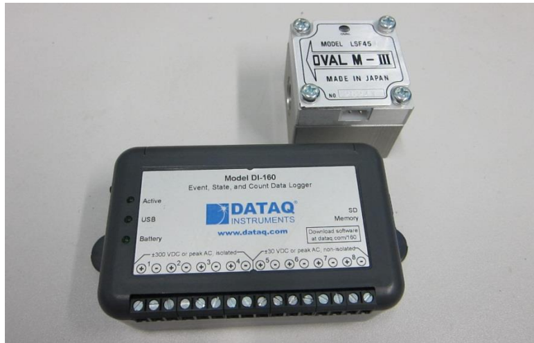
Photo 4.13. Fuel flow sensor with count data logger
