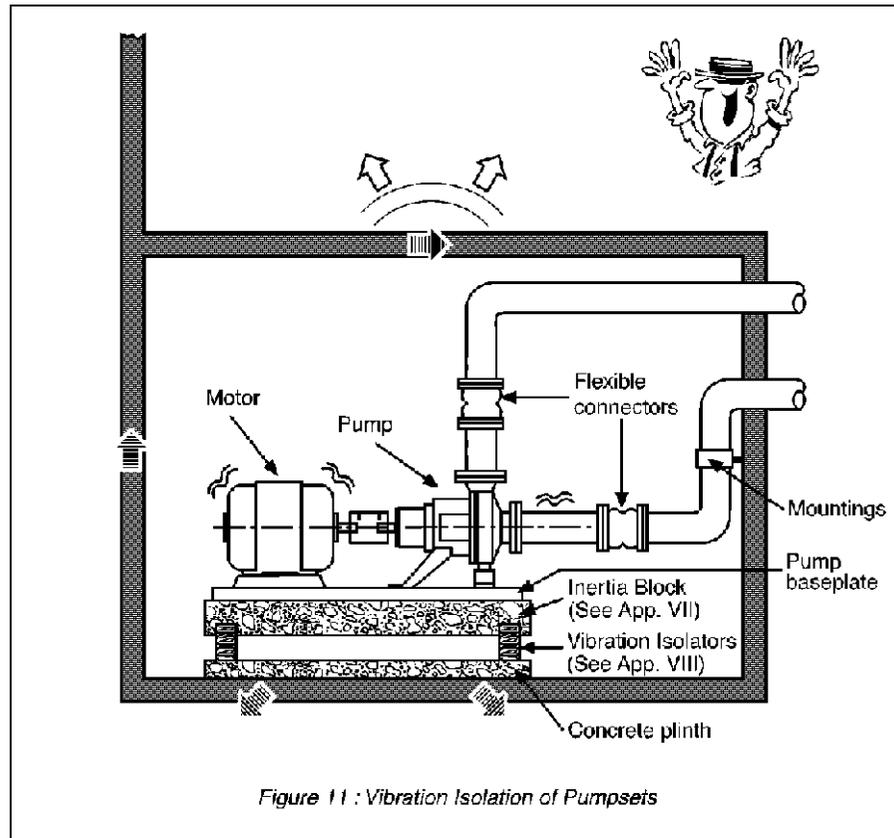
Figure 11 : Vibration Isolation of Pumpsets
