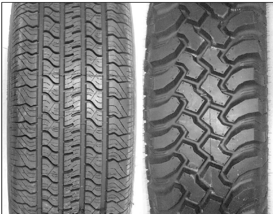
Fig. 14. Two tyres suitable for use as temporary "reference tyres" in the CPX trailer developed at the Hong Kong Polytechnic University. The left one is the ASTM Standard Reference Test Tire (SRTT) (new version) and the right one is the Goodrich MudTerrain tyre. The ASTM tyre is intended to respond to road surfaces typical of a car tyre, whereas the MudTerrain tyre is intended to respond to road surfaces typical of a truck tyre.
