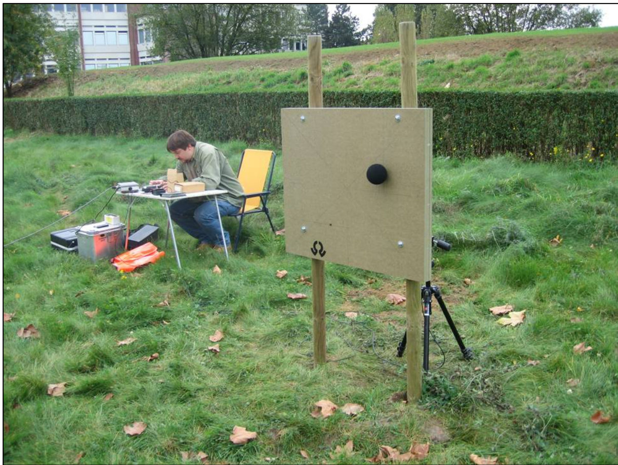
Fig. 12. Example of backing board used by the Belgian Road Research Centre [Goubert, 2006].
