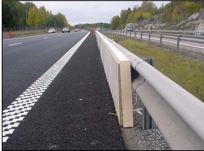
Fig. 16. Example of covering acoustically reflecting material with 100 mm mineral wool mounted in 2.4x1.2 m wooden frames, at the occasion of an SPB measurement (measurements in 2005 by VTI in Sweden). The SPB microphones were located at the far left roadside.
