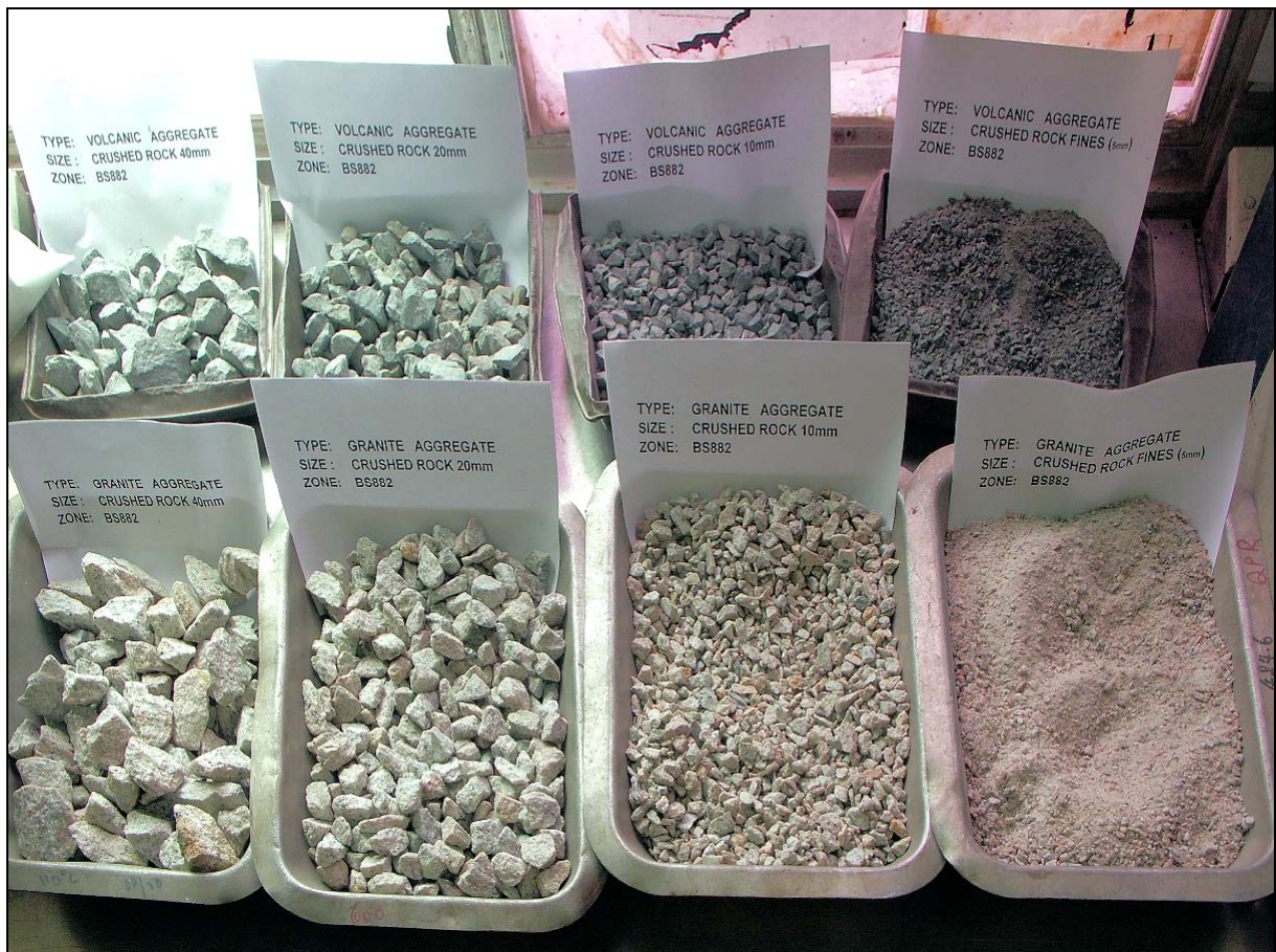
Fig. 22. Aggregate fractions and materials typical of Hong Kong. From the left: 40 mm, 20 mm, 10 mm, and 5 mm and less. The upper row is volcanic, the lower is granite.
