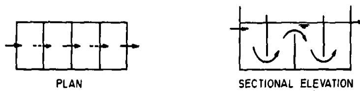
UP AND OVER BAFFLING FOR DEEP TANK
