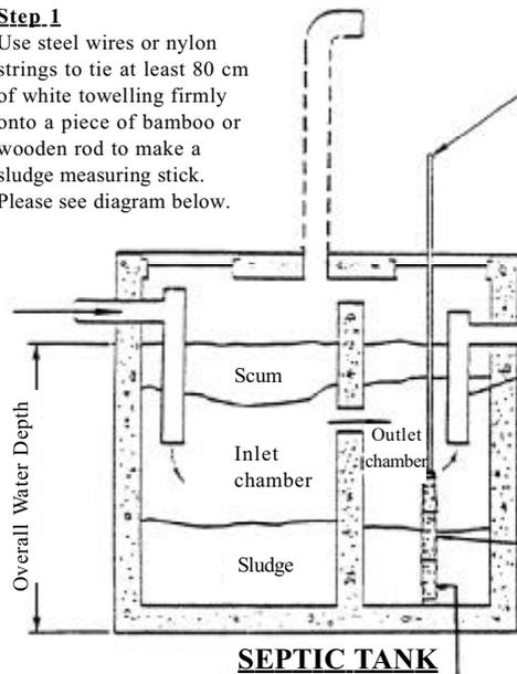
The soakaway pit and soil would be clogged very easily if solids were allowed to be carried into the soakaway pit; this would happen if sludge were allowed to build up to within 30 cm (1 ft.) of the bottom of the outlet tee pipe or if the outlet tee pipe were broken.
