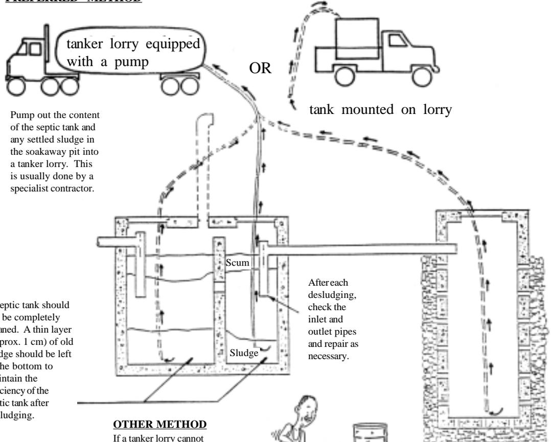
A septic tank should not be completely cleaned. A thin layer (approx. 1 cm) of old sludge should be left at the bottom to maintain the efficiency of the septic tank after desludging.
