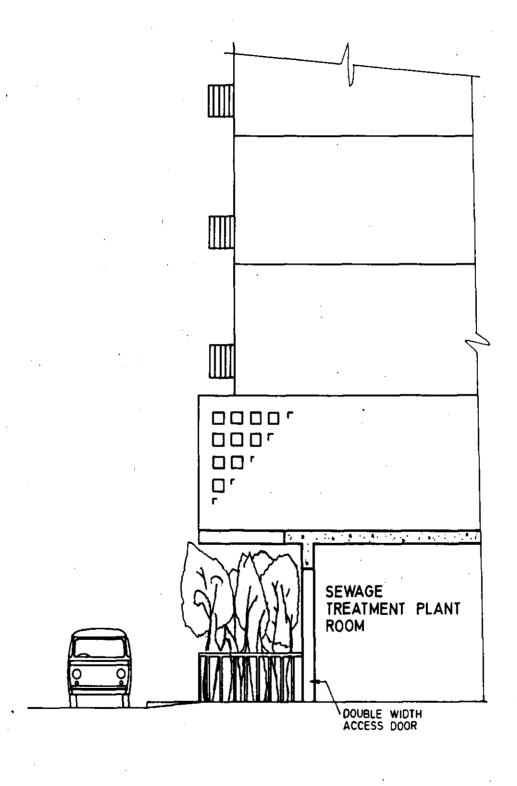
FIG. 1 GOOD VEHICULAR ACCESS AND PROPER ENTRANCE TO A SEWAGE TREATMENT PLANT
