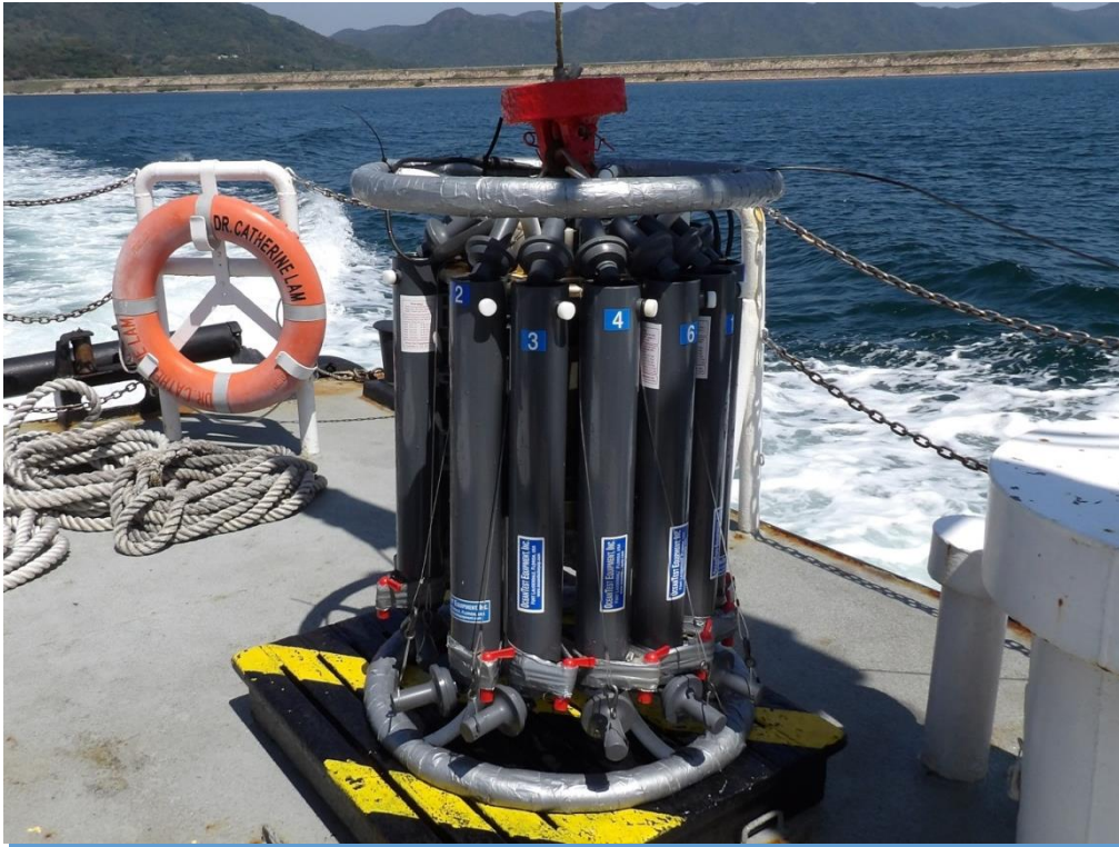
The water sampling process using a computer-controlled rosette water sampler.
