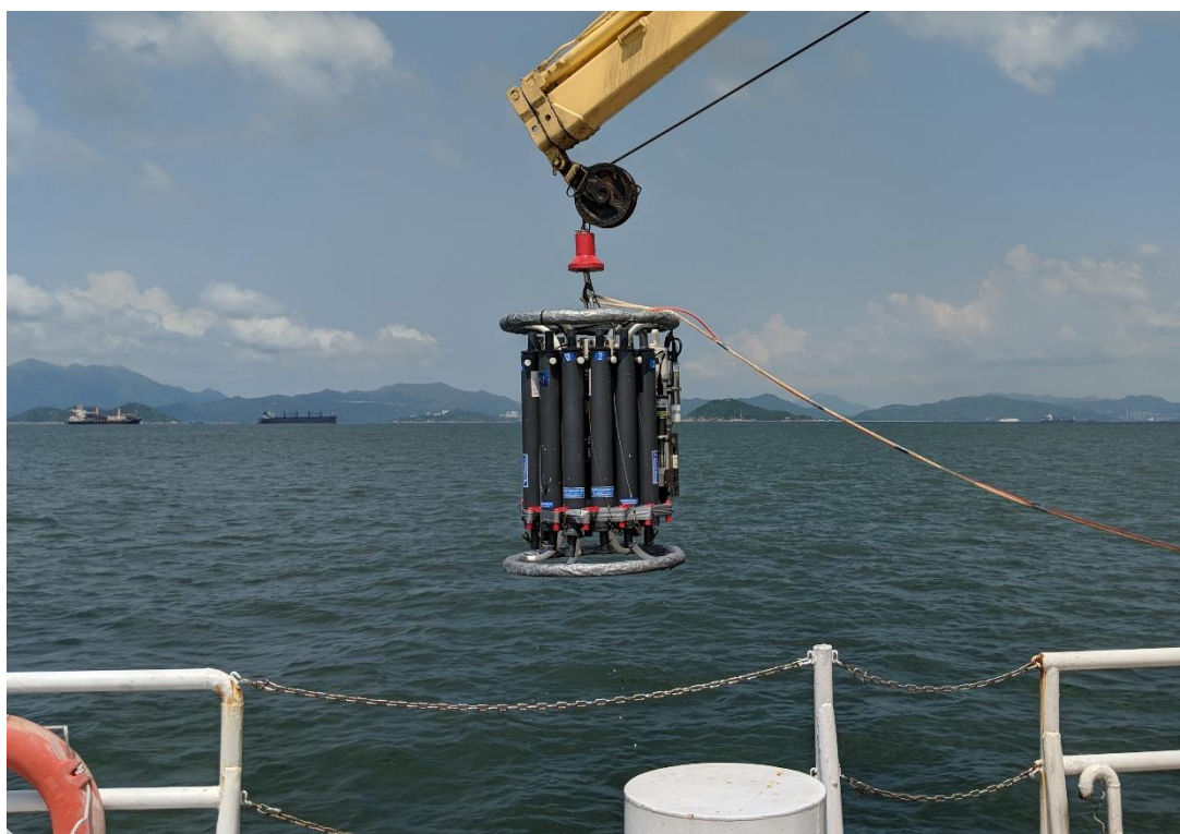
The computer-controlled rosette water sampler.
