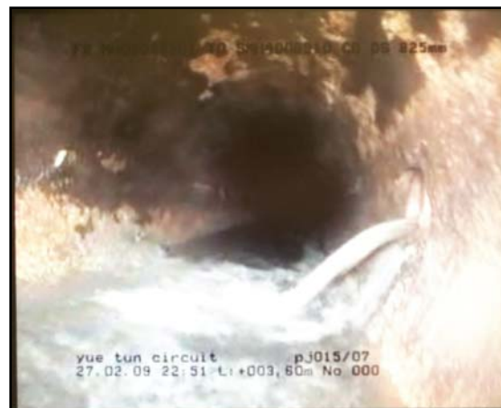
Photo 5 – Cross connection identified by CCTV method
