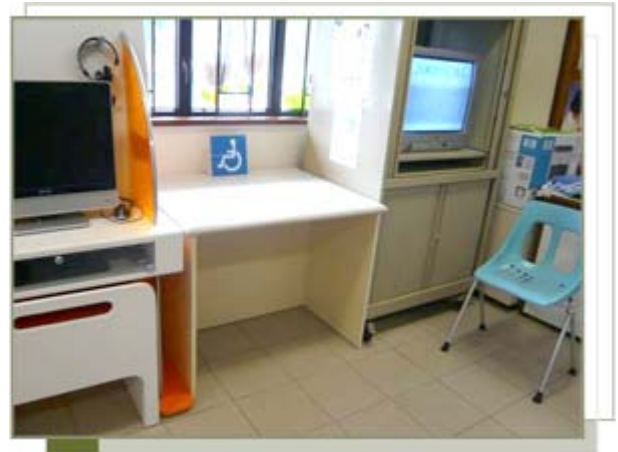
Desk with knee space and movable chair accommodates the needs of different users
