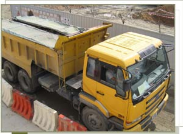
Dump truck equipped with a mechanical cover to prevent fugitive dust emission
