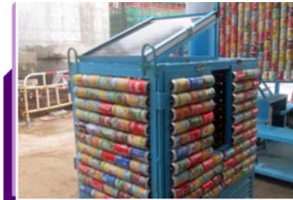
Moveable drinking water cabinet with solar panels
