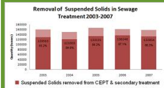
Removal of Suspended Solids
