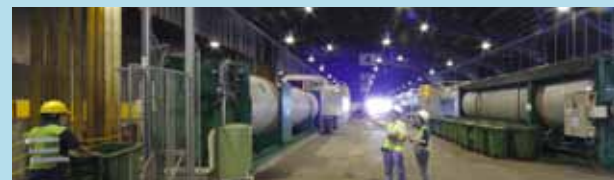
Upon completion of pre-treatment, all food waste goes to composting units for composting.
