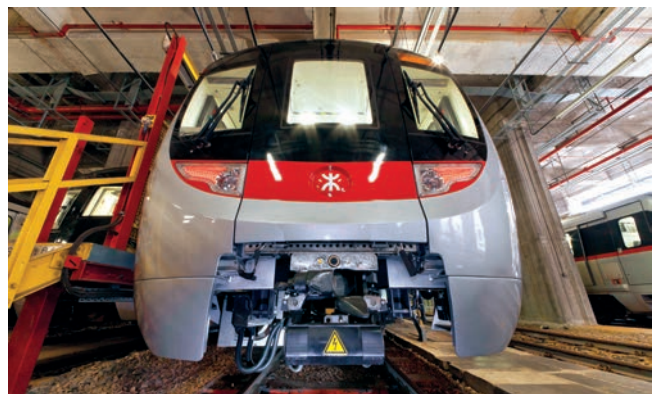
C-列車逃生門設於列車頭尾兩端。 Detrainment door is located at the front and rear of the C-Trains.
