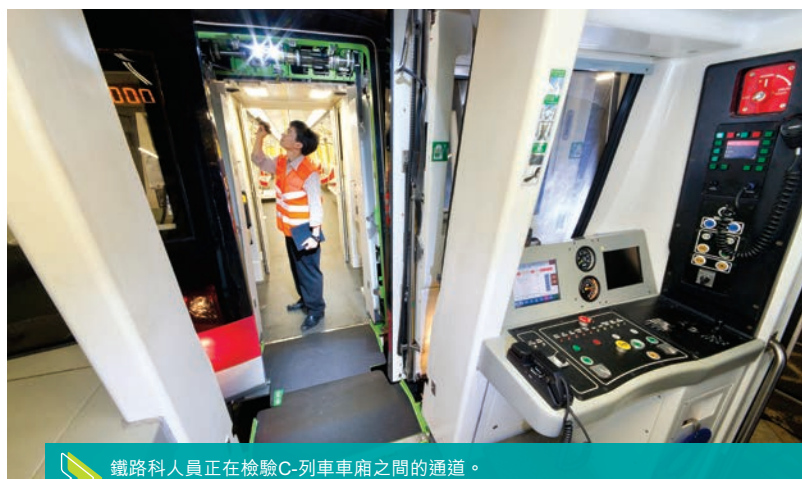
鐵路科人員為港鐵C-列車測試逃生門。 Railways Branch staff testing the detrainment doors of the MTR C-Trains.
