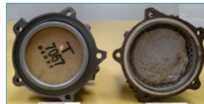
A brand new catalytic converter (left) and a used catalytic converter with deposits from vehicle engine exhaust (right).
