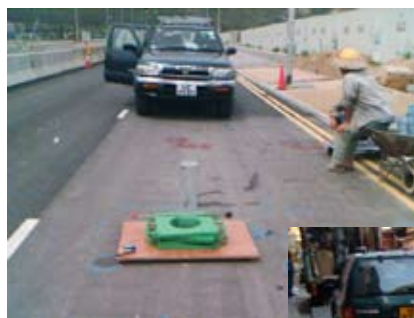
Drainability Test - for measuring hydraulic conductivity
