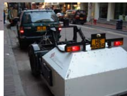
Close Proximity Method (CPX) - for measuring road/tyre noise level
