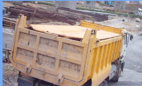
Dump truck fitted with automatic cover
