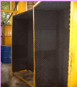
Use of enclosure for noisy road works
