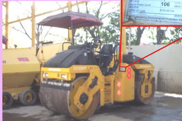
Use of Quality Powered Mechanical Equipment – typed vibratory roller
