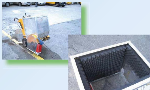
Winning Design for reduction of noise generated from a saw cutting machine
