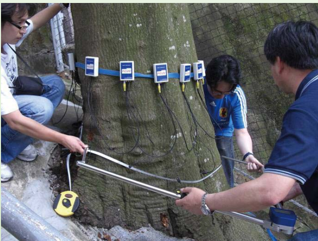
Tomographic testing in progress
