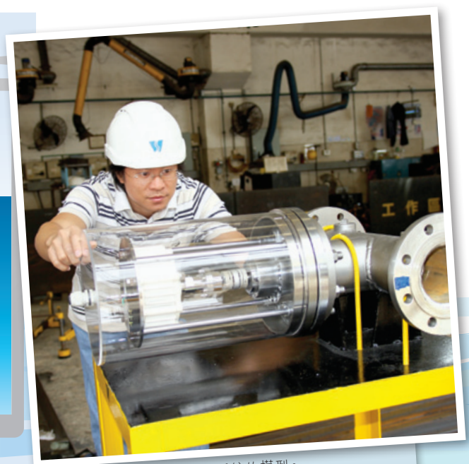
內聯閉式水力發電系統的模型。 A model of an inline hydroelectric generating system operating in confined conditions.
