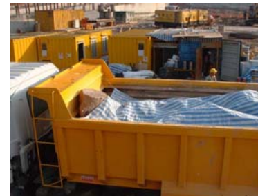
Cover is provided to dump truck before leaving the site, after checking of trip ticket
