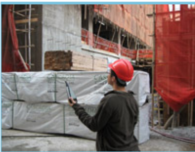
Site environmental monitoring for noise
