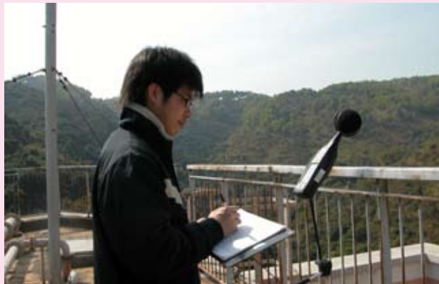
Staff was verifying noise data at a noise monitoring station.
