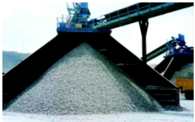
循環再造設施儲存的再造石料 Stockpile of Recycled Aggregates at Recycling Plant
