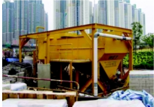
污水排出前先經沉積缸處理 Sedimentation Tank for Processing Waste Water before Discharge
