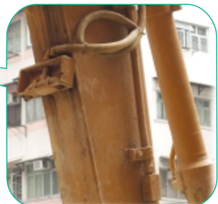
A good example of environmental practice by a contractor - the use of an excavator equipped with water spraying device to suppress dust emission during excavation
