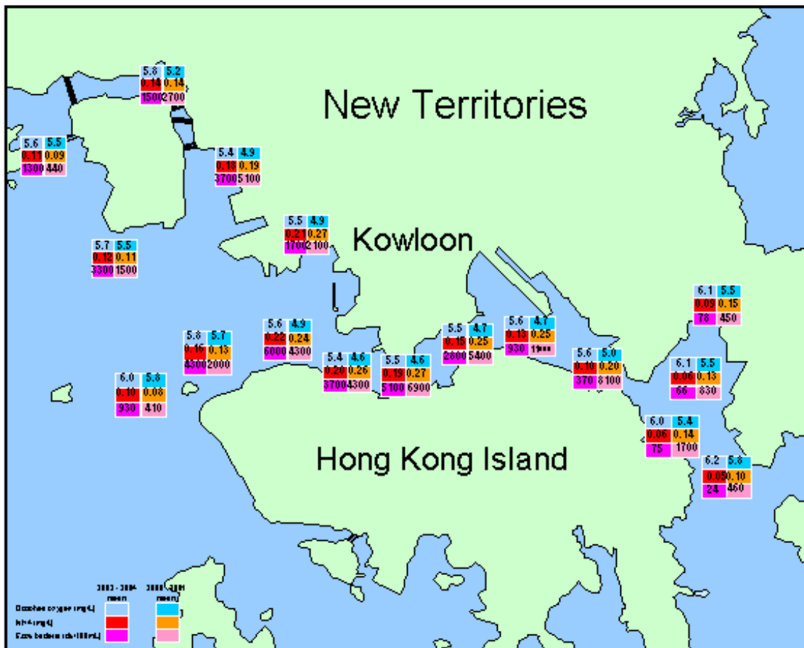
Map showing changes in dissolved oxygen (mg/L), NH 4 (mg/L) and E. coli bacteria (cfu/100mL) at 17 stations in the HATS enhanced monitoring programme between (2002 - 2004) and (2000 - 2001)
