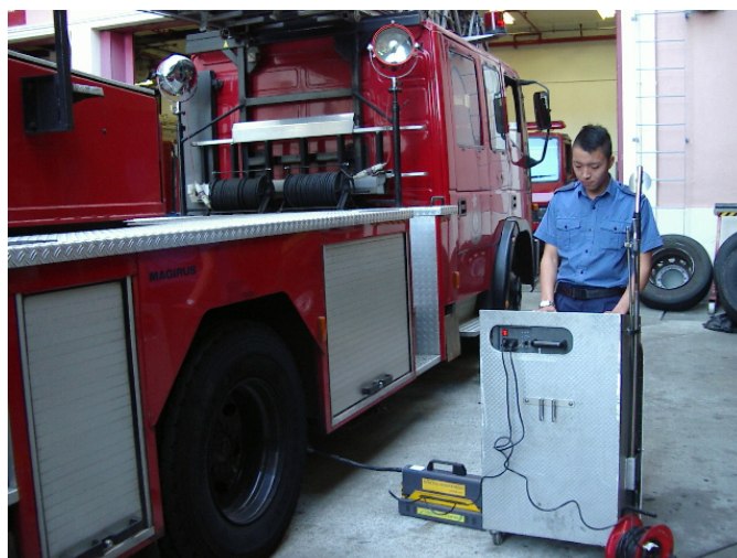
工程部屬員進行柴油氣車排放(黑煙密度)測試 Workshop staff Conducted Diesel Vehicle Emission(Smoke Density) Test
