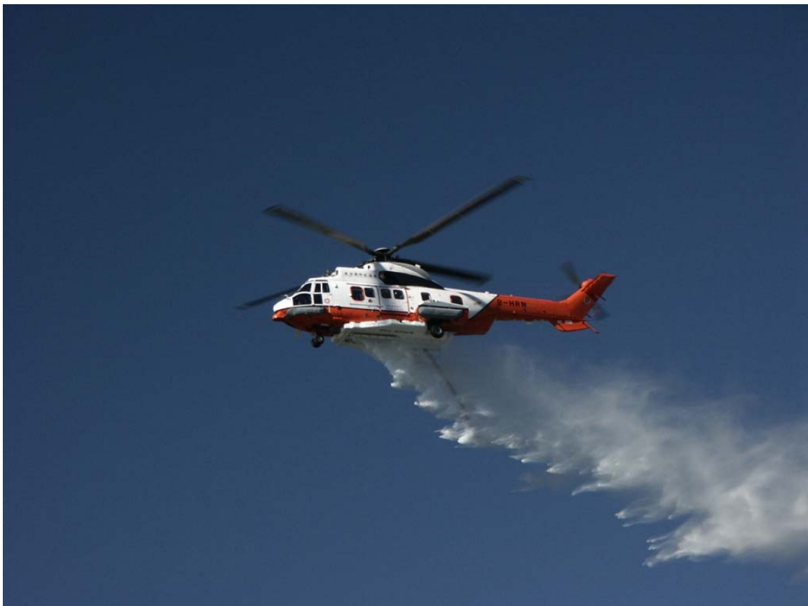
Helicopter in fire-fighting operation (fire tank)
