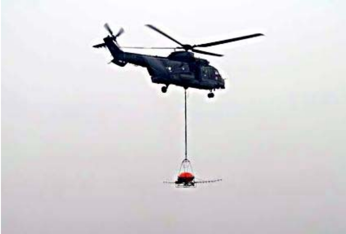
Helicopter in oil spill dispersant spray operation
