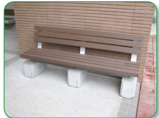
Benches made of recycled steel from the demolished hoarding and recycled concrete samples in Lam Tin Estate
