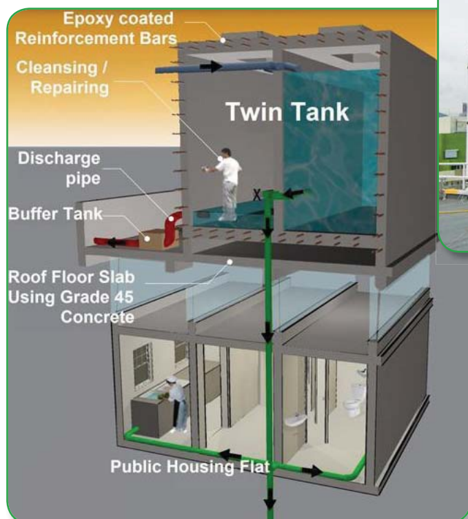
Interior design of the twin tank water supply system
