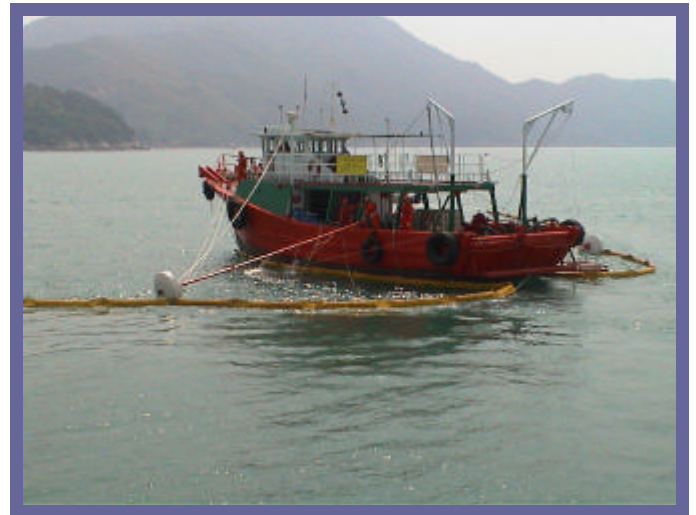
New Arrangement for Skimming Oil Spill devised by Contractor
