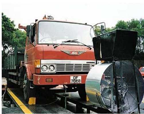
A goods vehicle being tested on a dynamometer
