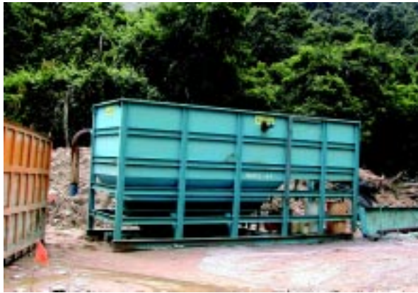
泥水在排放前經濕壕處理 Wetsep for muddy water treatment before discharge
