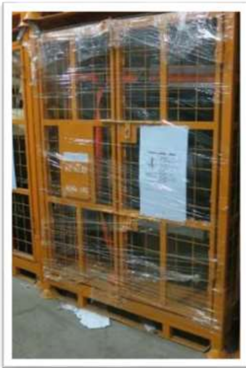
Figure 3 - Cage with plastic wrap and cover for containing waste monitors. Tray and catchment should be installed for receiving leakage/falling parts.
