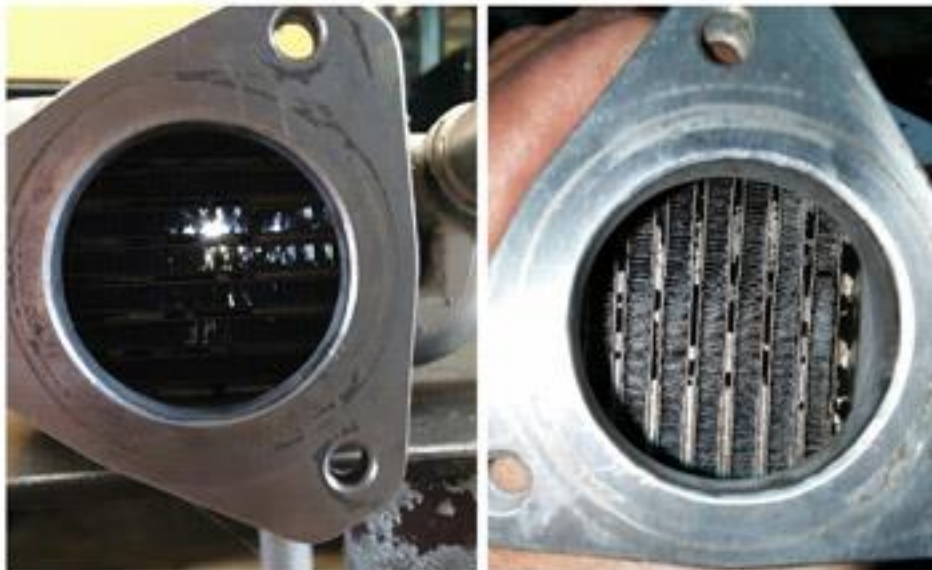
EGR Cooler after treatment with Cobra Clean
