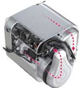
View from outside vehicle with reversing chambers
