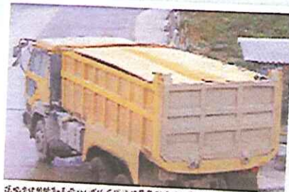
使用機械式車蓋以確保在運送建築廢料時不會散漏。 Use of mechanical covers on trucks for waste control during transportation of construction waste.
