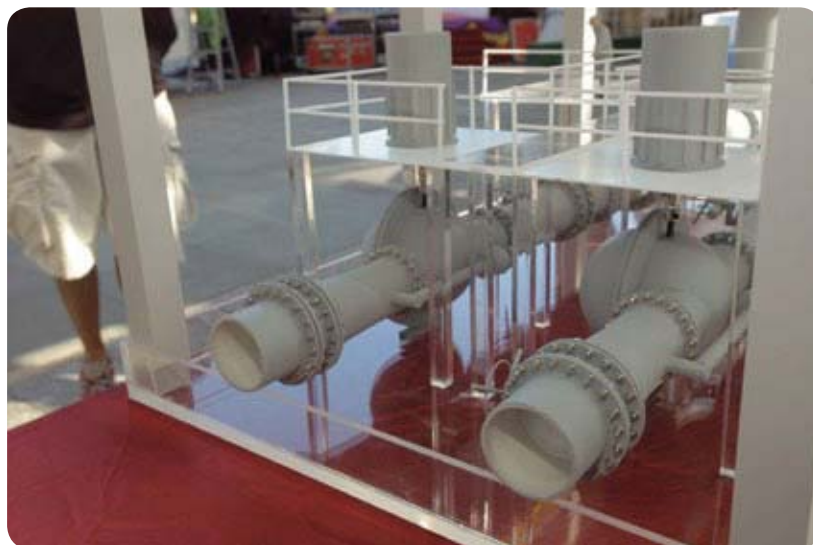
屯門濾水廠水力發電設施的設計模型。 The design model of a hydro-electricity plant to be installed at Tuen Mun Water Treatment Works.
