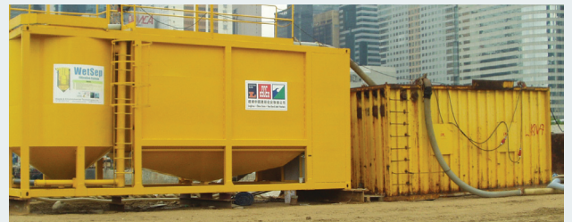
沉澱池處理工地上產生的廢水 Sedimentation tank to treat the wastewater generated on site
